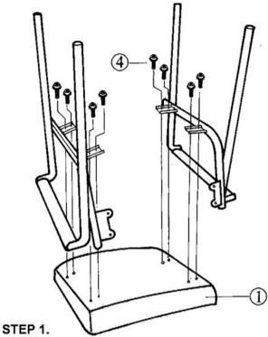
Align back of (1) seat to holes of (3) steel frame. Screw-in with (4) M6x20mm seat screw, but not making them too tight.
