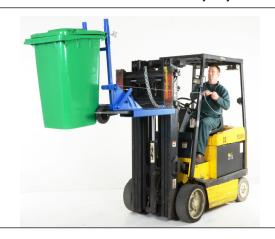
Step 8: Back away from the dumpster and adjust the elevation of the forks to prevent the cart from bumping against the wall of the dumpster. Once clear of the dumpster, lower the forks until the lid of the cart is just a few inches above the ground. Then, rotate the dumping mechanism back to the upright position. You should hear the latch lock (6) snap over the latch crossbar when the dumping mechanism is properly reset (see Parts Diagram and Bill of Materials on p. 3).
