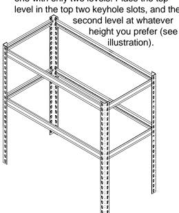
B. Instead of stacking the uprights on top of each other, as shown in step seven inside this sheet, place four shelf supports in the top two keyhole slots, being sure that the flat edge of each shelf support is facing up as described in earlier steps.
