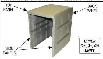
**Step 6.** If no optional sloping hood is ordered, install the three (3) filler strips into the recesses in the top panel of one (1) of the upper units. This will be the uppermost unit after the units are stacked.
