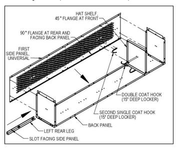
**Step 3:** Attach the second side panel and the right rear leg to the assembly of Step 2. On 15" deep lockers attach a third single coat hook. On 18" deep lockers substitute a single coat hook with a double bend for the third single coat hook and install the coat rod as shown on page 3. The locker chassis is now complete.
