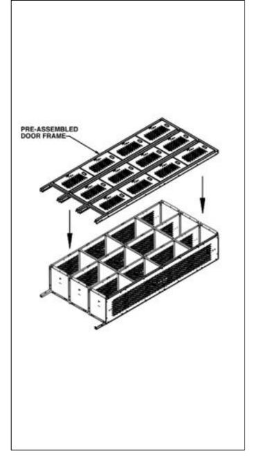
Step 9: Tighten all fasteners checking for squareness of the locker while tightening. Attach optional sloping hoods, end bases or front bases (see pages 4 and 5).
