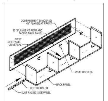
**Step 3:** Attach the second top shelf, the second bottom shelf, and an additional three coat hooks to the second back panel as in step 1.
