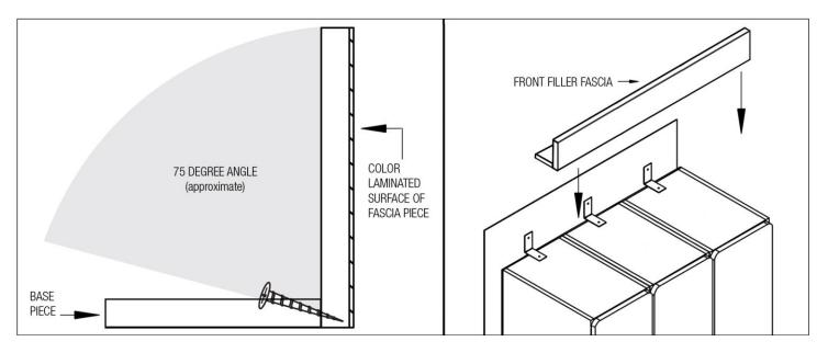
Align front of fascia with front edge of compartment (not the front edge of the door). Install the front filler fascia by fastening it to the lockers by installing screws from inside the lockers into the base of the front filler fascia. #8 x 1-1/4" long screws are provided for the installation.
