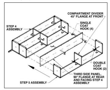
single coat hooks to the second back panel as in step 1.
