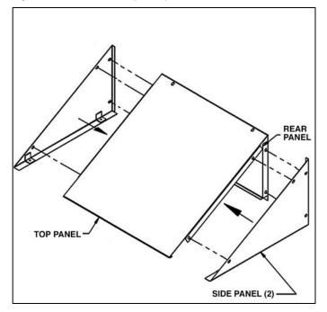
Step 3: Attach the sloping hood to the top of the locker with #10 - 24 x 3/8" slot less screws and #10 nuts (provided).
