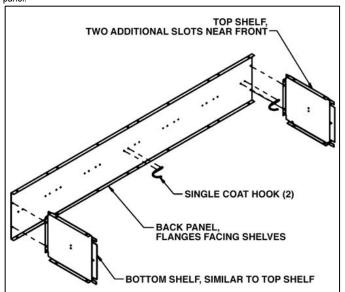
Step 1: Attach the top shelf, bottom shelf, and two single coat hooks to the back panel.
