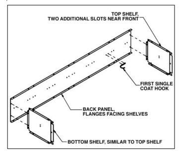
Step 2: Turn the back panel on its back with the shelves pointing upward. Attach the first side panel, the left rear leg, and the hat shelf to the assembly from Step 1. Attach a single coat hook with a double bend to accommodate the coat rod.
