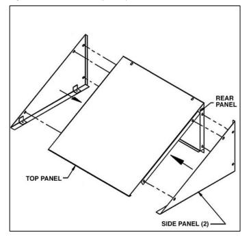
Step 3: Attach the sloping hood to the top of the locker with  $#10 - 24 \times 3/8$ " slot less screws and #10 nuts (provided).
