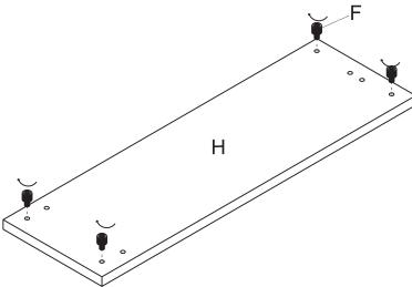
2 Use the Screw (E) to install the Top Panel (J) and Bottom Panel (H) to the Metal Frame (A&B), Use the Screw (E) to install the Shelves (I) on the Metal Frame (B), and Screw (D) to install the Shelves (I); Do not tighten screws until all shelves are aligned.
