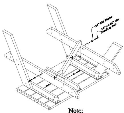
Leg is removed to show detail. Do not remove for this step.
