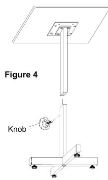
**Height Adjustment:** To adjust the height of the unit hold the inner tube with one hand and loosen the knob with the other hand. Set height at desired level and tighten knob.
