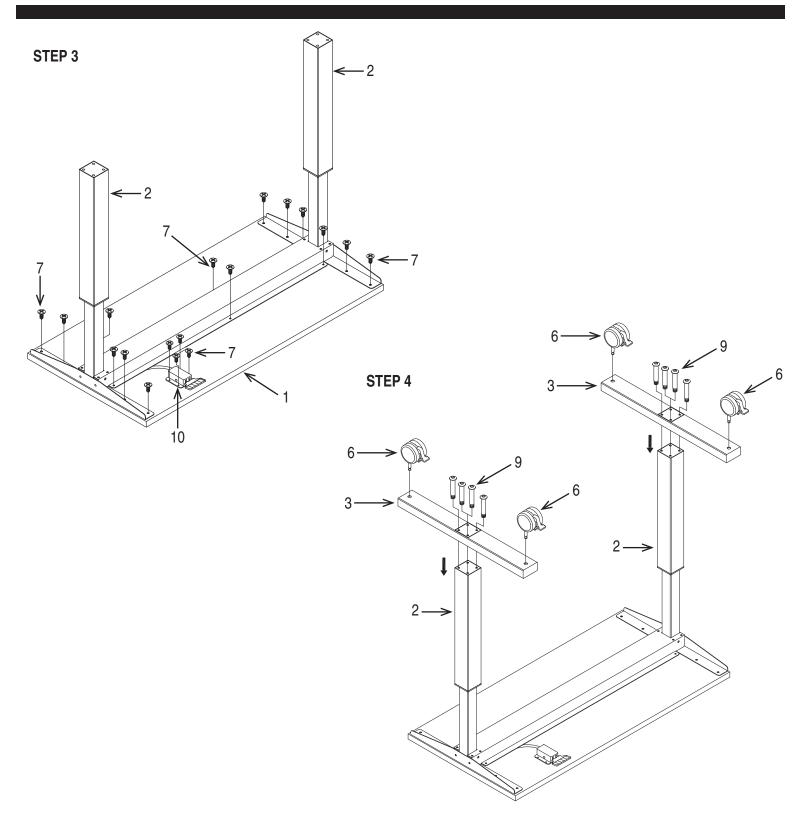
STEP 3 Attach Leg Post (2) assembly to Table Top (1) using fourteen Short Screws (7). FULLY TIGHTEN SHORT SCREWS (7). Attach Height Adjustment Lever (10) to Table Top (1) using four Medium Screws (7). FULLY TIGHTEN SHORT SCREWS (7).
