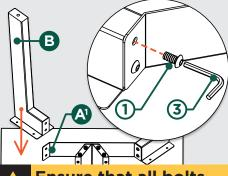
**Ensure that all bolts** are fastened tightly. To complete the Leg installation, secure each Leg B using four Pan-Head Screw (2) through the Leg Plate (B) to the Tabletop A.
