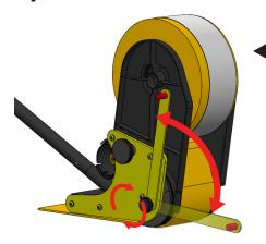
A guide arm can be adjusted with a small knob on the side of the Trolley. This will help ensure a stright, accurate line of tape.
