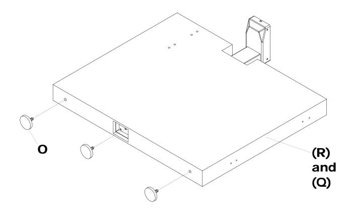
2 Insert Cams (A) into Fixed Modesty Panel (O). Install Cam Posts (C) into threaded inserts in Top of Legs (R and Q). Attach Fixed Modesty Panel (O) to Legs (R and Q) by turning Cams (A). Attach Stickers (B) over Cams (A).
