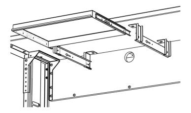
Insert keyboard tray into mounted slides.
