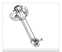
2. Insert the handle inserts and sensitive switch inserts of the harness 6.
