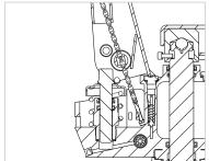
3. Put the chain through the hole on the shaft. With the handle at 45° tilt.
