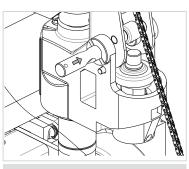
2. Push the handle shaft through the holes, fix it with the spring pin.
