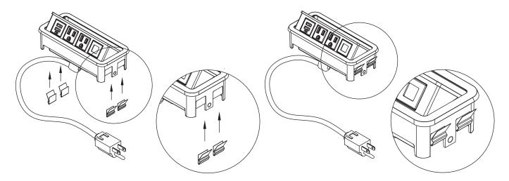
Attach 4 clips, two at each end on back of unit base.
