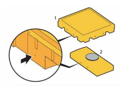
**Step 3:** Using the 2 3/8" hole saw, carefully place the drill bit of the hole saw in the center of the drill point and cut a hole through the sidewall.
