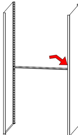
8. Place a shelf support at the rear of the unit in the bottom keyhole slots, in the same way you placed the shelf support in steps 4 through 6. Then, place a second shelf support at bottom front of unit.
