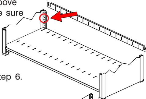
11. Continue the assembly by placing supports, shelves and backstops as described in steps 8 through 10. The recommended spacing between shelves is twelve inches, which equals six open keyhole slots between supports.
