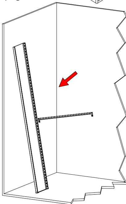
6. **PLEASE NOTE:** To firmly seat shelf supports and backstops, make sure both rivets are fully inserted in the keyhole slots, and firmly seated in the bottom of the slot. A rubber mallet can be helpful in accomplishing this. **Supports are not fully seated unless you can see an open space through the hole in the shelf support as shown below.**
