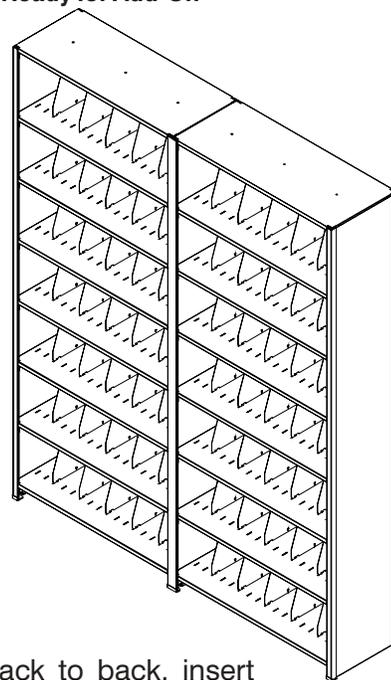
16. If installing units back to back, insert clothespins (Ref. No. 7) through top of uprights to tie units together.
