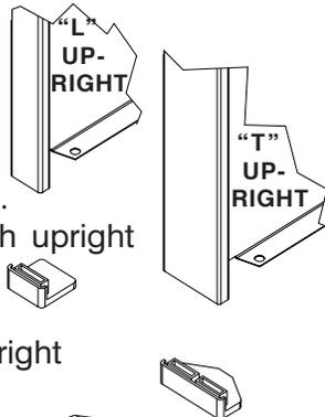
4. After determining which end of the upright is the bottom, attach a plastic foot (Ref. No. 8 or 9) to the bottom of each upright by pressing it into place. Note the difference at right between a foot for an "L" upright and a foot for a "T" upright.
