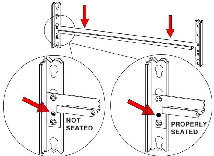
7. Hold a second "L" upright (or a "T" upright if you are assembling multiple units) approximately 36" away. Pull the first upright away from the wall using the shelf support you attached in step 3, and insert the other end of the shelf support into the second upright. **NOTE: Take care not to let the uprights fall, as they are not stable until step 7 is completed.**
