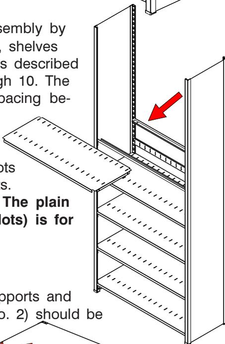
12. The top shelf supports and top shelf (Ref. No. 2) should be installed flush with the upright top. Note that the top shelf has no divider slots.
