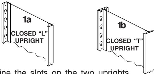
3. Examine the slots on the two uprights you have selected. When an upright is standing up on end, the narrow part of the keyhole slots should be toward the floor, while the wide part should be toward the top.
