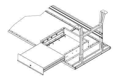
**2.** Attach the drawer assembly to the WBSR-xx using eight 1/4-20 x 1/2 bolts. Close drawer and turn workbench back over to the upright position.
