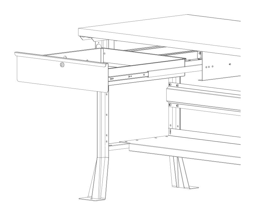
**4.** Cycle the drawer in and out a few times to check operation.
