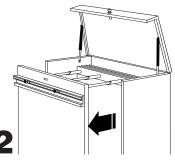
When filing or retrieving, roll the drawer out of the main cabinet to a point where about two inches of the pins remain in the posts of the cabinet.
