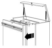
When selected drawings are on the pins, roll the entire drawer away from the cabinet as far as it will go, disengaging the pins from the posts.
