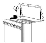
Insert the Drawing Selector behind the desired drawing so the notches ride on cabinet posts. Use the Selector to move the groups of drawings from posts to pins.
