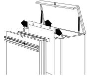
The space between pins and posts permit filing or removal without rubbing on adjacent drawings. Remove drawings from the side or the top. Always handle by carrier strips – not drawings. Drawings transfer to posts when cabinet is closed.
