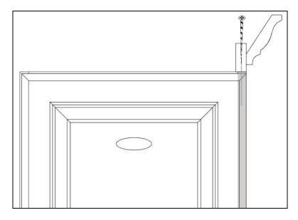
When installing crown molding placed at the front of the locker, open the door and use three to four screws to attach the molding to the locker from the underside of the top of the locker and into the crown molding as shown below.
