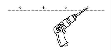
Care should be taken to mount the units. Units should be mounted to wall studs using correct fasteners. Failure to do so may result in collapse of the unit and subsequent personal injury. Mounting hardware not included. Mounting hardware used should be based on wall material. Consult an installation professional for proper wall mounting.
