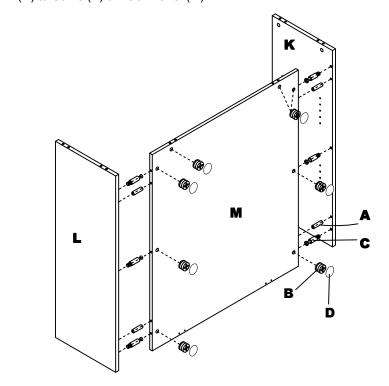
2 Insert Wood Dowels (A) into Side Panels (K & L). Insert Cam (B) into Side Panel (K & L). Install Cam Posts (C) Top(J). Attach Top (J) to assembled cabinet by turning Cams (B). Apply Cam Stickers (D) to Cams (B) of Side Panel (K &L).
