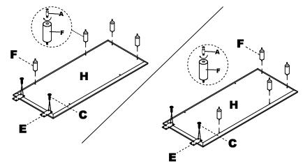
(I) and Side Panel (J). Place Top (H) onto Modesty Panel (I) and Side Panel (J). Place Top (H) onto Modesty Panel (I) and Side Panel (J) and lock in place by turning Cams (B). Apply Cam Stickers (D) to Cams (B) of Modesty Panel (I) and Side Panel (J).
