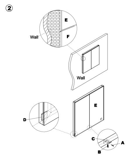
Place foam spacer (D) at white line on the backside of the presentation board prior to attaching bracket (C). Attach the Mntg Bracket (C) to the bottom of the presentation board using screw (B) then attach the bracket to the wall using screw (A).
