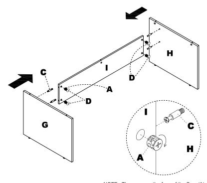
NOTE: The arrow on the face of the Cam (A) should point towards the Cam Post (C) for proper alignment.
