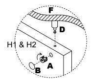
NOTE: The arrow on the face of the Cam (A) should point towards the Base Stand-off (D) for proper alignment.
