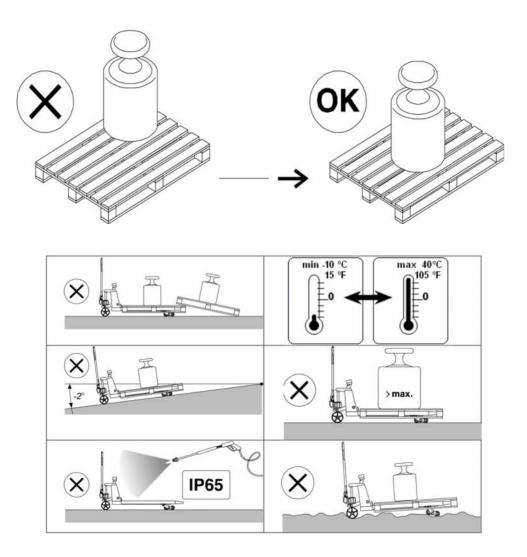
Fast temperature changes should be avoided because condensation may form in the electronics. During acclimatization the indicator must be turned off.
