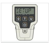
1. Press "U" key and "T" key simultaneously for Setup mode in normal mode.
