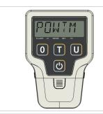
5. Press the "U" key to skip the "power -off time setting"
