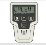
6. Make sure that here is no cargo on the frame, and Press "T" key to confirm calibration.
