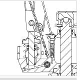
3.Put the chain through the hole on the shaft.
