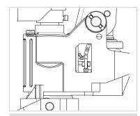
4. Fix the chain in the slot of the unloading plate.
