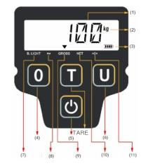
Figure 2-1 Operating panel in Normal Weighing Mode
