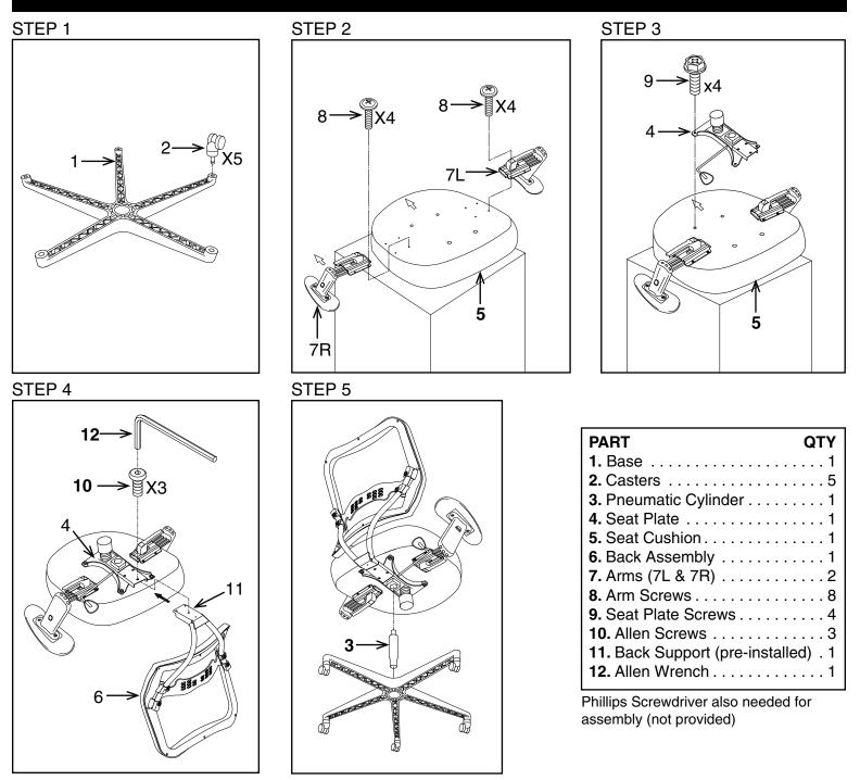
Remove all parts from carton, separate by part numbers indicated on parts list, and verify part quantities.
